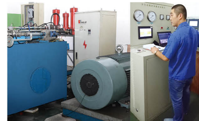
电机功率250KW 转速3000r/min 超大功率叶片泵全自动测试平台 Full automatic testing platform for vane pump with motor power of 250KW speed of 3000r/min
